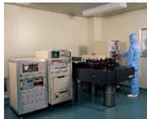
Iodine absorption stabilized He-Ne (633 nm) laser for length measurement
