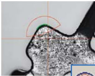
One-Click Arc Tool This tool is appropriate for capturing an arc and the radius of a corner.
