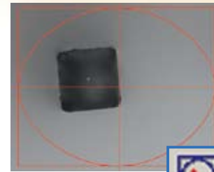
Area Centroid Tool This tool evaluates the position of a feature's centroid. It is appropriate for positioning a different feature.
