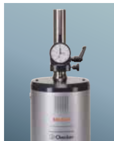
Inspection using analog type indicator
