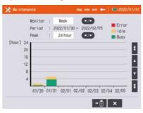
Operation log data is retained for up to 2 months, and can be output to a USB memory device.
