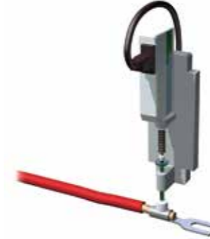
5 Measurement of crimping height
