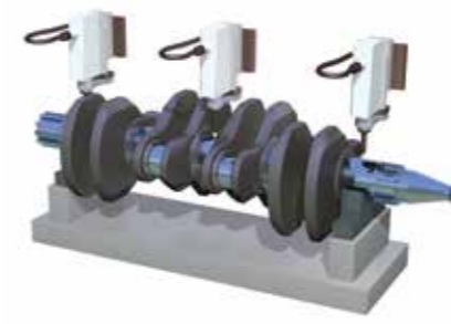
7 Workpiece runout measurement
