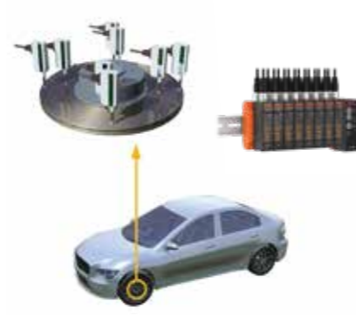
2 Brake disk multipoint measurement
