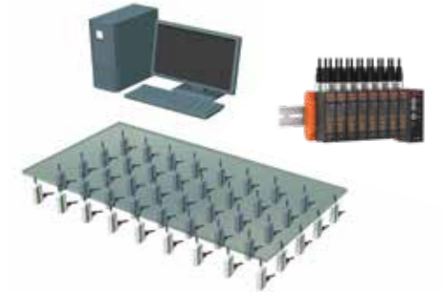
6 FPD board multipoint measurement
