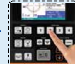
Press the [CONDITION (setup recall)] button, as needed.
