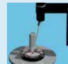
Bring the detector into contact with the workpiece.
