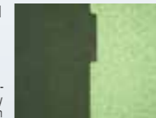
Measurement of the width of micro-recessed-forms cannot be accurately performed due to low magnification
