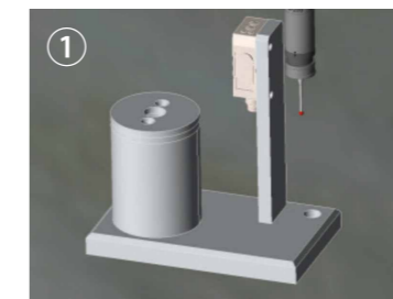
The probe moves to the sensor of the stylus cleaner.
