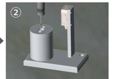
The probe moves to above the cleaner.
