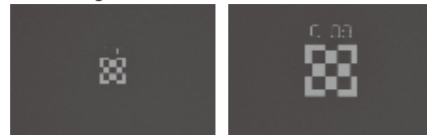
Turret 1x Field of view: 2.49 x 1.86 mm Turret 2x Field of view: 1.24 x 0.93 mm
