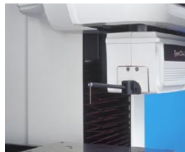
Wide range detector employing active control technology
