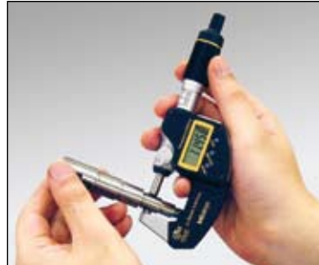
Measuring coaxial workpiece
