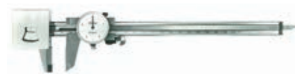
Figure 120 Mitutoyo Constant-force Dial Caliper for Plastic, 1973
