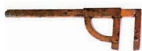
Figure 81 Shiga, Nagahama, Kyubei Kunitomo's hereditary brass sliding calipers
