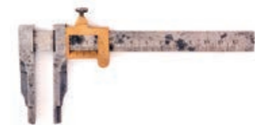
Figure 40 Vernier Caliper (Made in France) (Measuring range: 100 mm, Minimum reading: 0.1 mm), Around 1890
