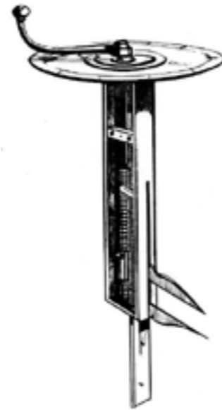
Figure 10 Gascoign's Screw-operated Microscope Caliper (UK), 1639
