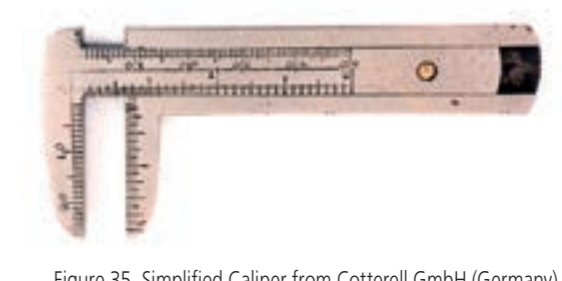
Figure 35 Simplified Caliper from Cotterell GmbH (Germany) (Measuring range: 2 in, 50 mm, Graduation: 1/16 in, 1 mm) 1930
