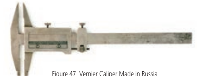
Figure 47 Vernier Caliper Made in Russia (Measuring Range: 150 mm, Minimum reading: 0.05 mm (dividing 39 mm into 20) 1910
