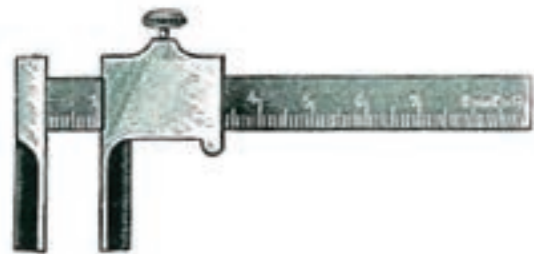
Figure 16 Adolf Phifer Trading Company's Simplified Calipers (Measuring Range 65 mm) 1905
