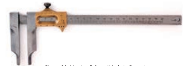
Figure 39 Vernier Caliper (Made in France) (Measuring range: 150 mm, Minimum reading 0.05 mm by dividing 19 mm into 20), Around 1890
