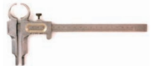
Figure 41 Vernier Caliper with Round Jaws (Made in France) (Measuring range: 150 mm, Minimum reading: 0.1 mm), Around 1890
