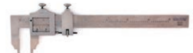
Figure 48 Vernier Caliper from Brown & Sharpe Mfg. Co. (Measuring Range: 5 in, Minimum reading: 0.001 in.) 1910
