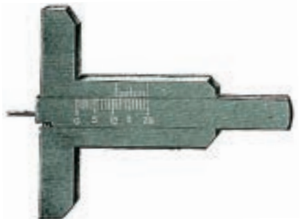
Figure 68 Depth gage from Adolf Pfeiffer (Germany) (Measuring range: 10 mm, Minimum reading: 0.1 mm) 1905
