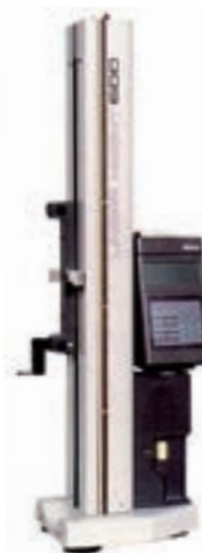
Figure 134 Mitutoyo Digital Height Gage (Linear Height LH) Resolution: 0.001 mm, Stroke: 600mm, 1998
