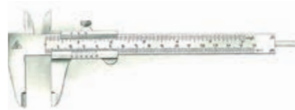
Figure 62 Pocket Vernier Caliper from Carl Mahr Esslingen a. N. (Germany) (Measuring range: 120 mm, 5 in, Minimum reading: 0.05 mm, 1/128 in) 1931
