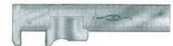
Figure 22 Sliding Caliper from Brown & Sharpe Mfg. Co. (United States) (Maximum scale: 4 in, Graduation: 1/32 in) 1924
