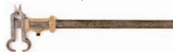
Figure 92 Fujiyama Mfg. Co. Round-jaw Ordinary-type Vernier Caliper, 1944
