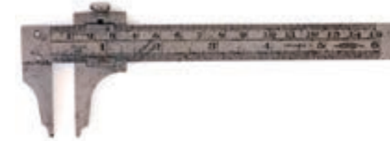
Figure 36 Simplified Caliper from Sheffield (UK) (Measuring range: 5 in, 13 cm, Graduation: 1/32 in, 0.5 mm) 1950
