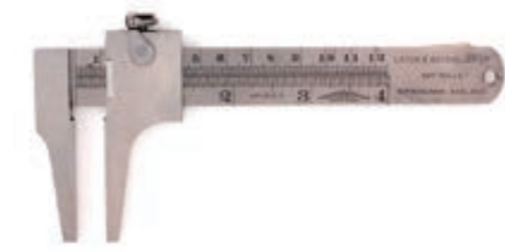
Figure 32 Simplified Caliper from Chesterman Sheffield (UK) (Measuring range: 4 in, 120 mm, Graduation: 1/32 in, 0.5mm) 1900
