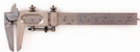
Figure 42 Multi-purpose Vernier Caliper from Rawco Co. (UK) (Provided with a depth bar, Maximum scale on lower edge: 120 mm, Upper scale: 5 in, Measuring range: 100 mm, 4 in, Minimum reading: 0.1 mm, 1/128 in (dividing 7 graduations over 1/16 inch into 8) 1900
