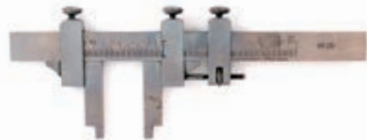
Figure 25 Sliding Caliper from L.S. Starrett Co. (United States) (Measuring range: 3~6 in, Graduation: 1/64 , 1/100 in) 1890, 1927
