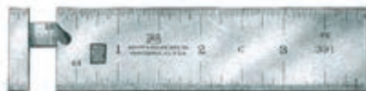
Figure 17 Brown & Sharpe Mfg. Co. (United States)-made Simplified Calipers (Maximum Scale Value 4 in, Scale Interval 1/32, and 1/64 in) 1924
