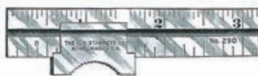
Figure 19 The L. S. Starrett Company (United States)-made Rule with Thumb Slider (Maximum Scale Value 6 in, Scale Interval 1/8, 1/16 in) 1927
