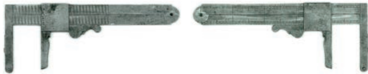
(b) Reverse-side sun graduations. Minimum reading is 5 rins, and maximum graduation value is 5 suns
