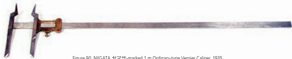
Figure 90 NIIGATA ヤマサ-marked 1 m Ordinary-type Vernier Caliper, 1935
