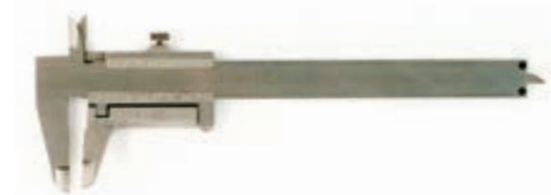
Figure 59 Swivel Jaw Caliper from Helios Co. (Germany) (Measuring range: 5 in, Minimum reading: 1/128 in, 1/1000 in) 1940
