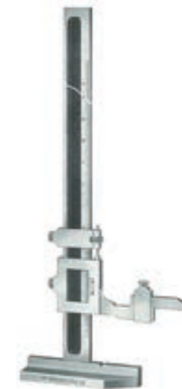
Figure 74 Brown & Sharpe 18 in Height gage (United States) (Graduation 1 / 1000 in) 1924
