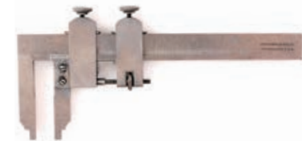
Figure 23 Simplified Caliper from Brown & Sharpe Mfg. Co. (United States) (Measuring Range: 3 in, Graduation: 1/32 in) 1910, Same type in 1924
