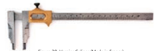
Figure 38 Vernier Caliper (Made in France) (Measuring range: 150 mm, Minimum reading 0.1 mm by dividing 9 mm into 10), Around 1890
