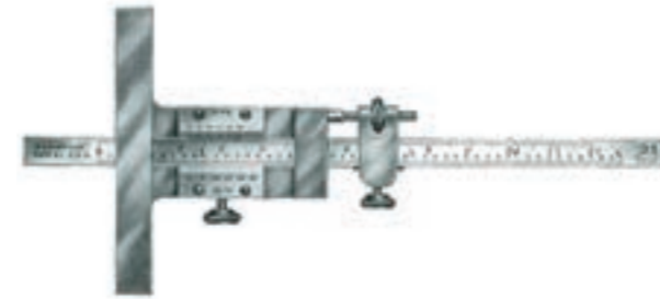
Figure 70 Depth gage from Brown & Sharpe (United States) (Measuring range: 3 1/2 in, 88 mm, Minimum reading: 1/64, 1/1000 in, 0.02 mm) 1924
