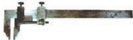
Figure 50 Caliper from L.S. Starrett Co. (The main scale has 1/40 inch graduations and the jaw feeding screw has 25 graduations over its circumference to provide a minimum reading of 1/1000 inch.) Around 1900
