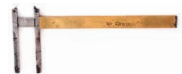
Figure 9 Scabbard Type Sliding Caliper, Simplified Nogisu (in Units of inch and mm) (Made in France), about 1870
