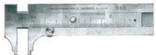
Figure 18 Brown & Sharpe Mfg. Co. (United States)-made Simplified Calipers (Maximum Scale Value 3 in, Scale Interval 1/32 in) 1924
