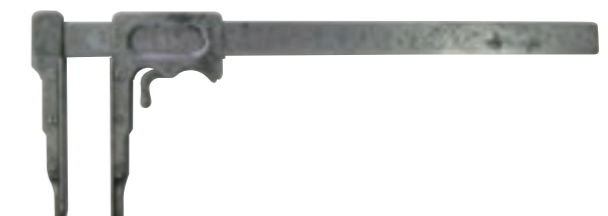
Figure 57 Outside Vernier Caliper (Holland) (Measuring range: 6 in, 120 mm, Minimum reading: 1/128 in, 0.1 mm) 1920
