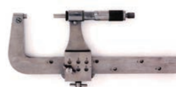
Figure 56 Caliper with Movable Micrometer Head from L.S. Starrett Co. (United States) (Measuring range: 6 in max.) 1920
