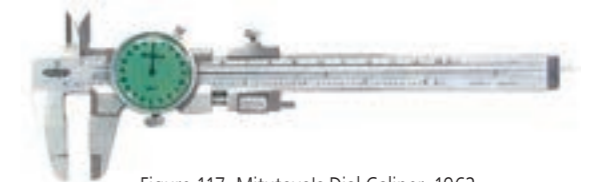
Figure 117 Mitutoyo's Dial Caliper, 1962
