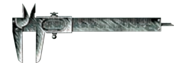
Figure 45 Multi-purpose Vernier Caliper from Adolf Pfeiffer (Germany) (Provided with a depth bar, Named Columbus Caliper, Measuring range: 100 mm, 4 Zoll, Minimum reading: 0.1 mm, 1/128 Zoll) 1905
