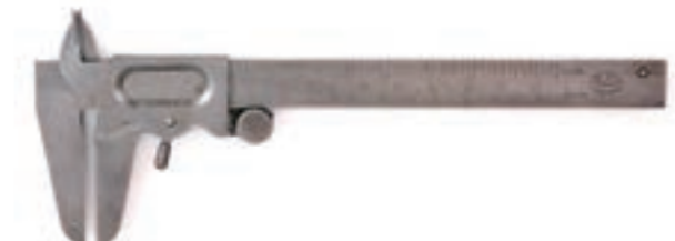
Figure 58 Vernier Caliper from Helios Co. (Germany) (Measuring range: 120 mm, 4 in, Minimum reading: 0.1 mm, 1/128 in.) 1920
