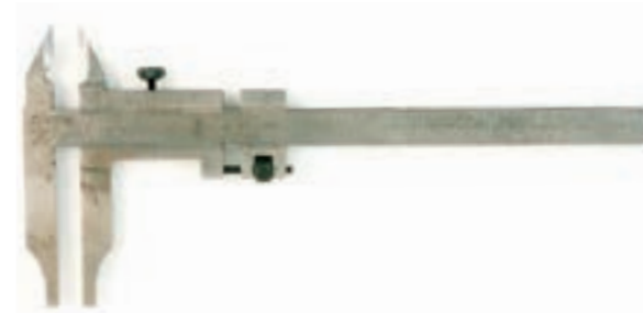
Figure 66 Vernier Caliper with Brand Logo of CES (Germany) (Measuring range: 5 in, Minimum reading: 1/1000 in) 1940
