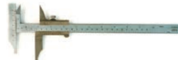
Figure 98 Multipro Inc. (German-made) Offset Vernier Caliper, 1967
