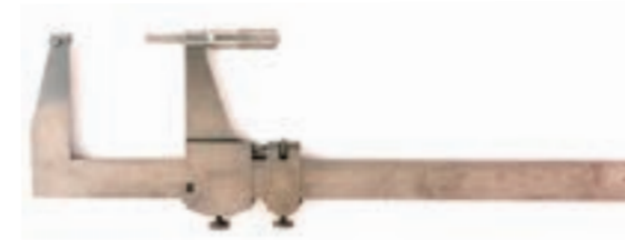
Figure 55 Caliper with Micrometer Head from Brown & Sharpe Mfg. Co. (United States) (Measuring range: 12 in max.) 1920
