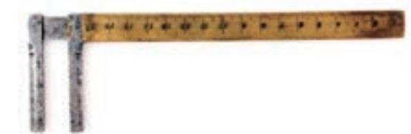
Figure 8 Scabbard Type Sliding Caliper, Simplified Nogisu (in Units of inch and pouce) (Made in France), about 1840
