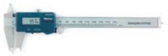
Figure 139 Mitutoyo Digital Caliper with Main Scale Graduations, 1987
