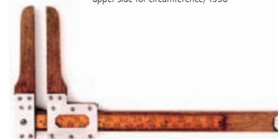
Figure 29 Wooden Sliding Caliper (Made in France. Upper graduation for diameter: 1 cm with maximum scale of 25 cm, Lower graduation for circumference: 2.5 cm with maximum scale of 80 cm) 1930
