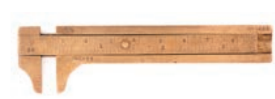
Figure 34 Simplified Caliper from Rabone and Sons (UK) (Measuring range: 3 in, 80 mm, Graduation: 1/32 in, 1mm) 1920
