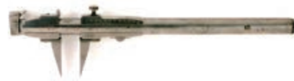
Figure 89 Ninken-made (Japanese) Round Bar-type Vernier Caliper, 1940
