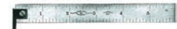
Figure 21 Rule with Hook from Brown & Sharpe Mfg. Co. (United States) (Maximum scale: 4 to 36 in, Graduation: 1/8, 1/16 in) 1924
