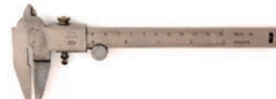
Figure 33 Simplified Caliper from Parker (UK) (Measuring range: 5 in, 130 mm, Graduation: 1/32 in, 1 mm) 1920
