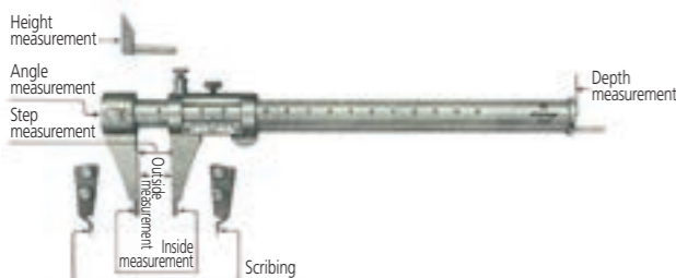
Figure 113 Mitutoyo Universal Vernier Caliper, 1970
