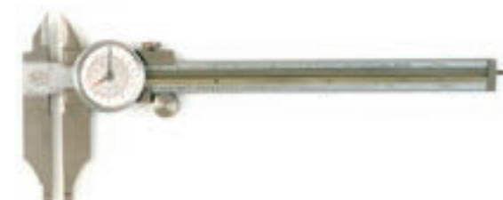
Figure 115 Helios Co. (Germany-made) Dial Caliper with a Dual Inch/Millimeter Indicator, 1960
