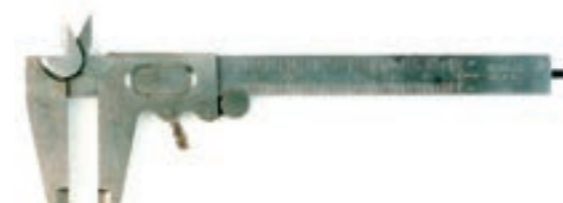
Figure 31 Simplified Caliper from Dunlop Co. (United States) (Measuring range: 5 in, Graduation: 1/16 and 1/32 in) 1920
