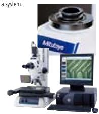
Digital Color Vision System DV-520 (Microscope main unit: MF-UB1010TH)
