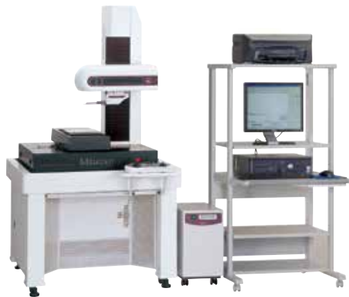
Surftest Extreme SV-3000CNC (With drive unit inclination mechanism)
