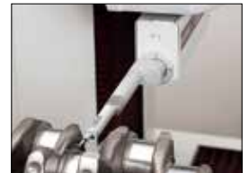
Measurement example for rotary-type detector holder (backward facing)
