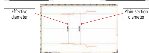
3. Continuous top-bottom measurement function
