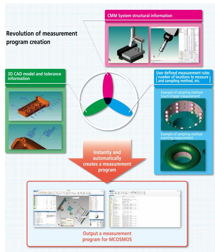
**FEATURES** Adding tolerance information<sup>\*</sup> to the 3D CAD model and clicking once are all it takes to automatically generate a measurement program with MiCAT Planner.
